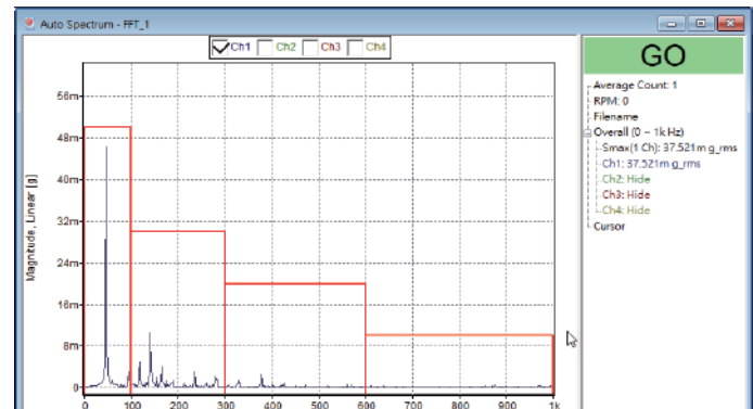
Overlay of band limit curve(s) on the spectral plot showing the severity of vibration or acoustic signals.
